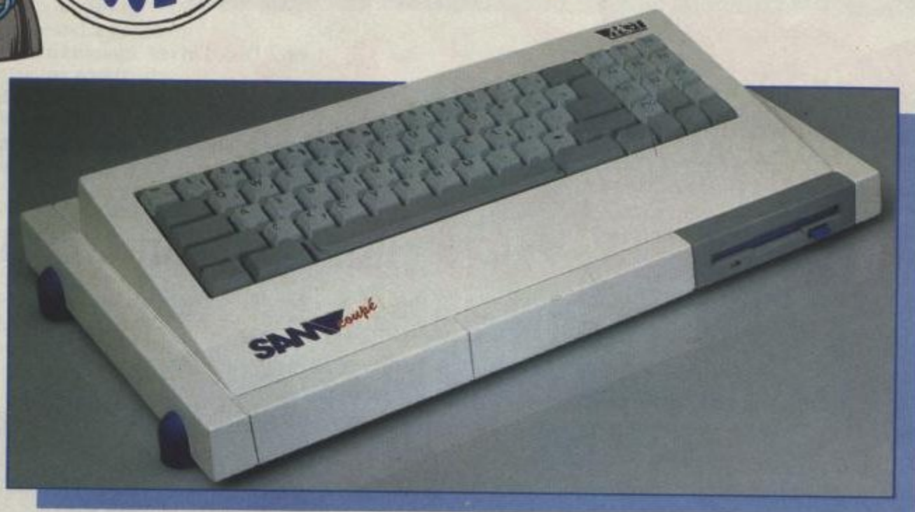
The Coupé's slot-in disk drive
