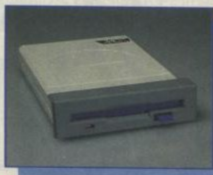
The Coupé's slot-in disk drive
